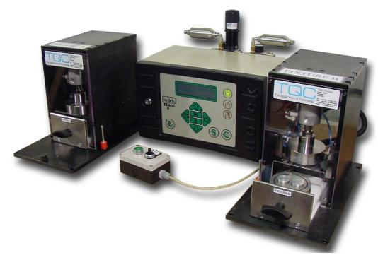
The system shown leak tests cartridges used in military applications as explosive bolts. It is important that the cartridges fire correctly in the critical applications where they are used. The cartridge must therefore not take on moisture which could affect the operation in service.
