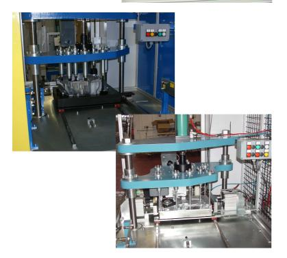
The key to successful leak testing is in the design and manufacture of the fixture and sealing system. TQC has many years experience of seal and fixture design and our expertise in this area enables us to engineer representative, reliable and repeatable leak test equipment.
