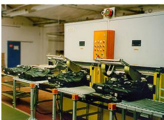
TQC provide complete leak test facilities utilising leak test instruments and pumping groups from Varian or Alcatel Vacuum Technology. The leak measurement resolution may
