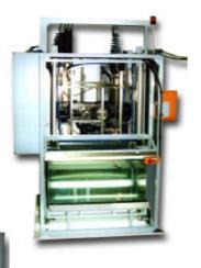
Water submersal or dunk tanks are a widely used method for location of leaks in complex assemblies and products with air bubbles present around the leaking area.
