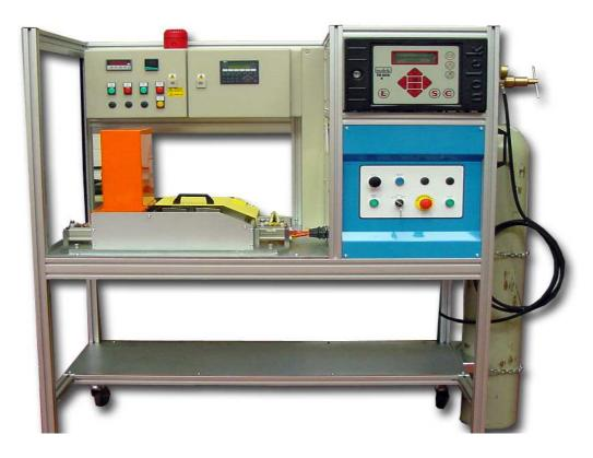
This piece of equipment has been designed and built to leak test an automotive fuel rail to a leak specification limit of 4mm<sup>3</sup>/sec at 3.5 bar.
