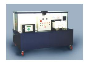
This machine combines TQC's experience of leak detection and automatic inserting. In the case of this machine, if the leak test fails, the automatic inserting process will not actuate.
