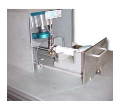
The machine was designed to leak test the inductance weld on a plastic shower head.
