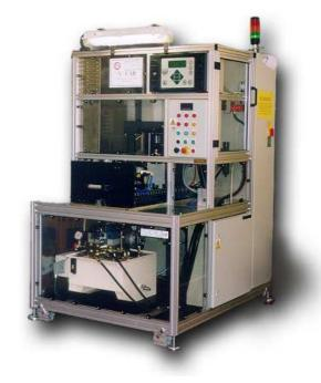
The facility is designed to carry out four automatic air decay leak tests on a manually loaded assembly. These leak tests are on the
